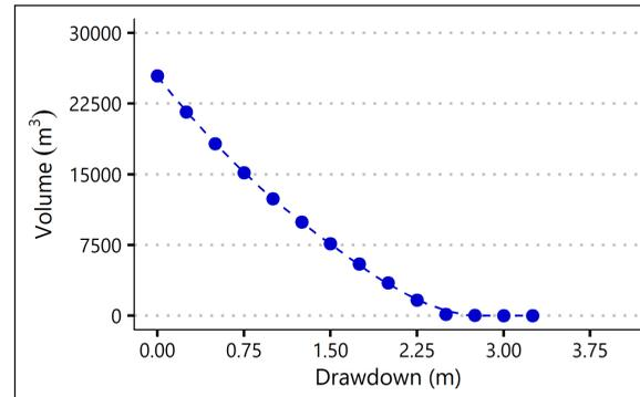
Water volumes are determined using detailed designs, as-builts, and/or volume tables when available. If design information is limited, then a bathymetric survey is used to measure pond volume. The decreasing relationship between volume at particular drawdown levels allows pesticide applicators to estimate volume quickly in the field immediately before treatment so as to achieve the desired concentration precisely.
